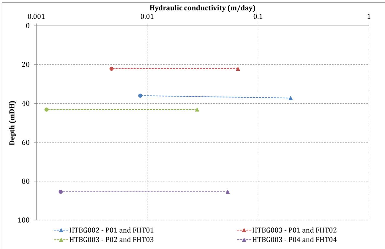
Note: circles represent packer test data and triangles represent falling head data
