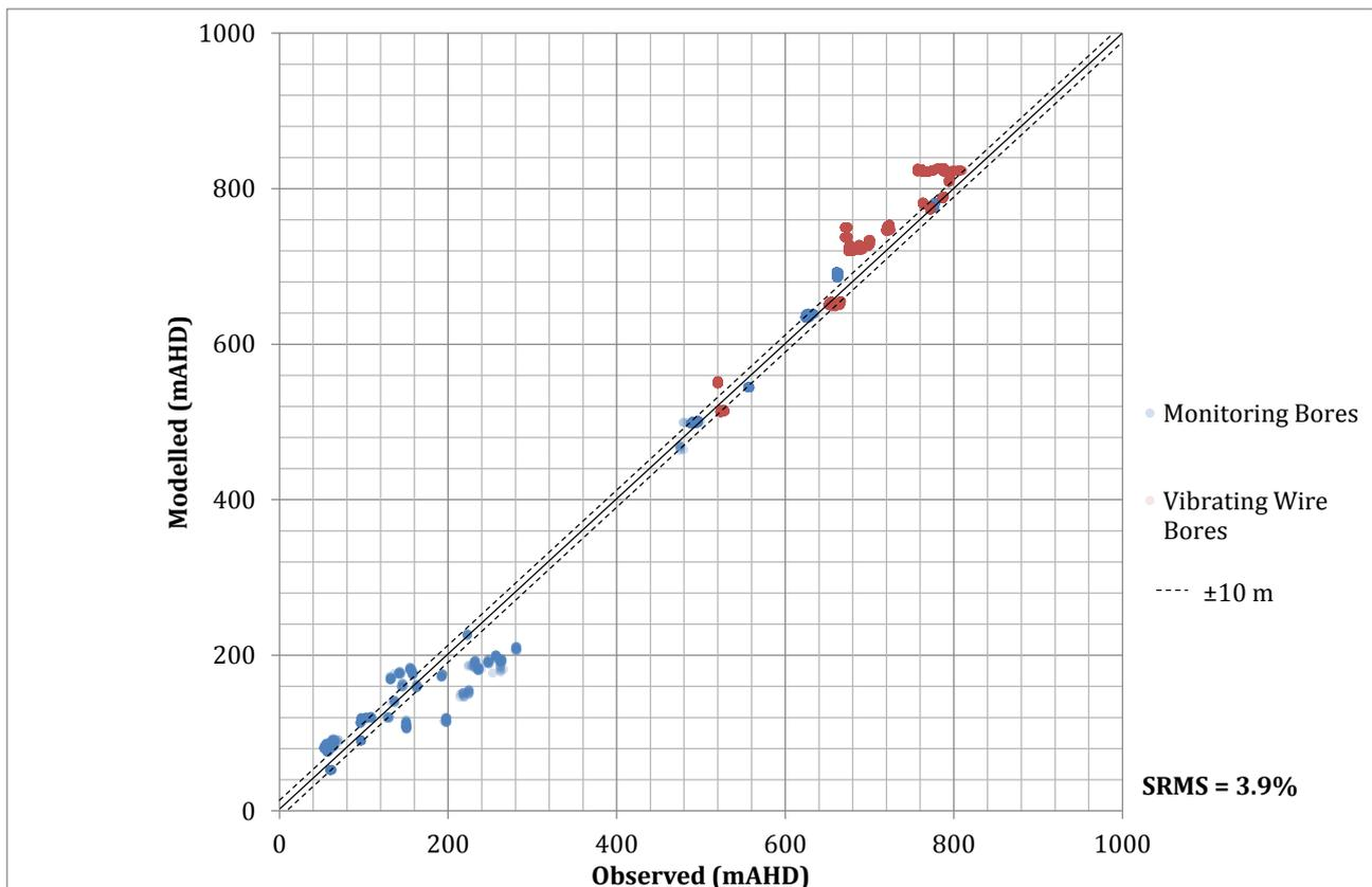
**Figure D 3.4 Transient calibration – modelled vs observed groundwater levels**
