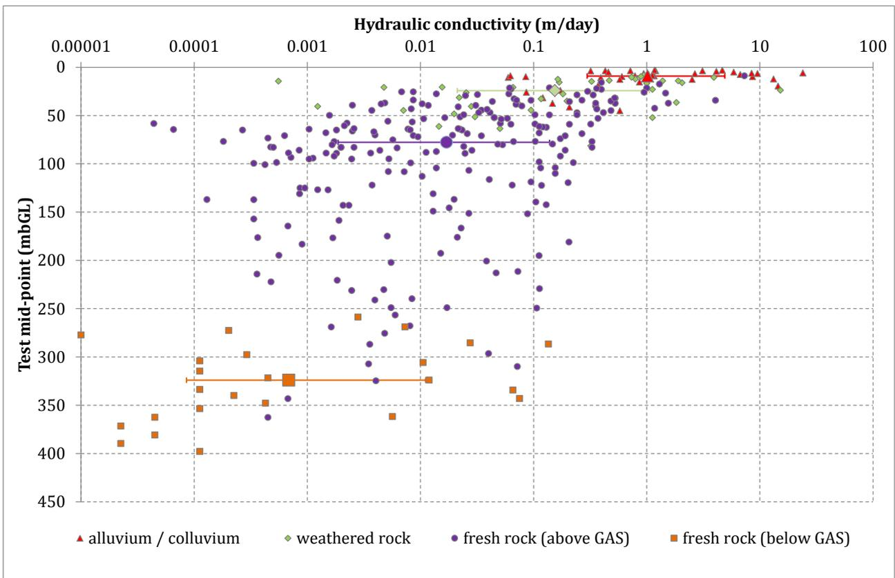
**Figure B 3.1 Hydraulic conductivity of each unit**
