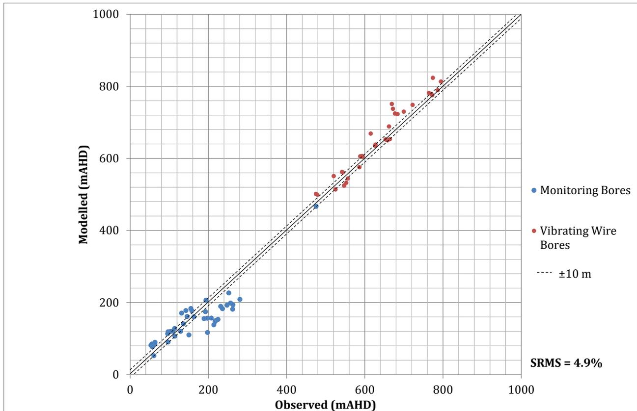
**Figure D 3.2 Steady state calibration – modelled vs observed groundwater levels**
