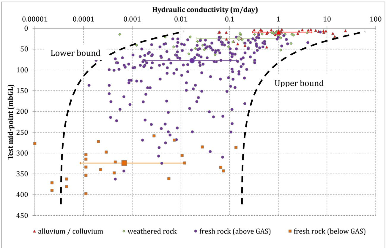
**Figure 4.9 Hydraulic conductivity with depth**
