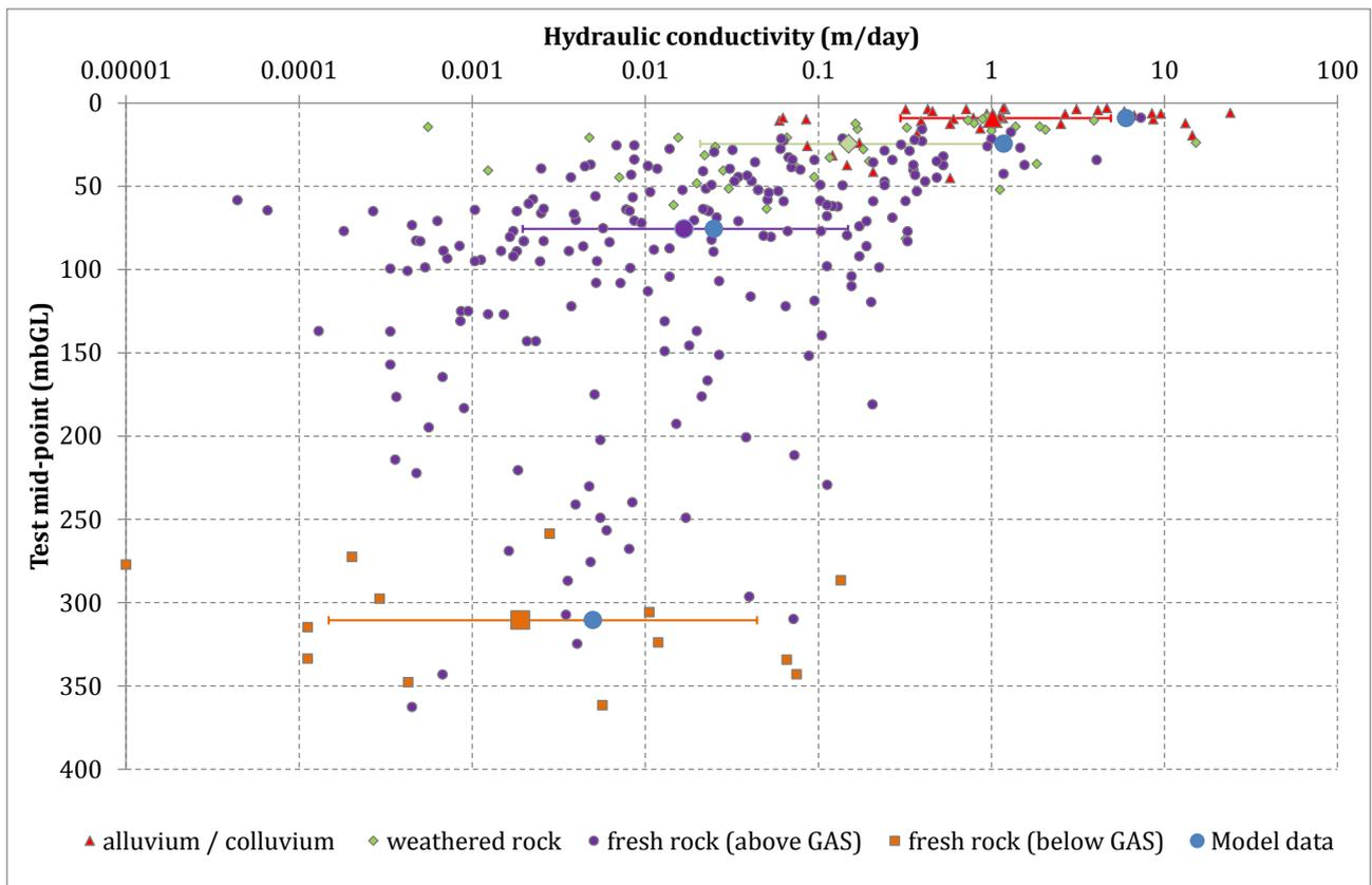
**Figure D 3.6 Hydraulic conductivity distribution graph**
