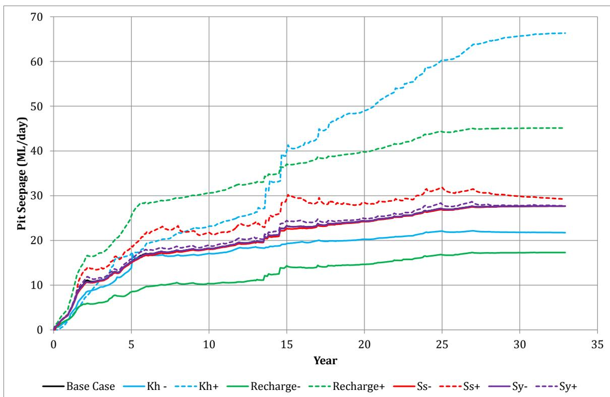
**Figure 6.7 Sensitivity - Predicted open-pit groundwater seepage**
