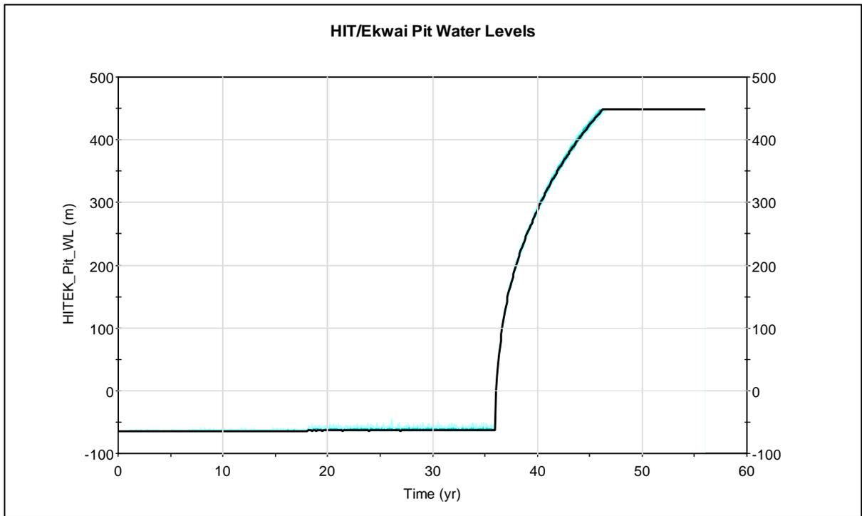
**Figure 4-9: HIT/ Ekwai pit inundation post closure – diversions maintained**
