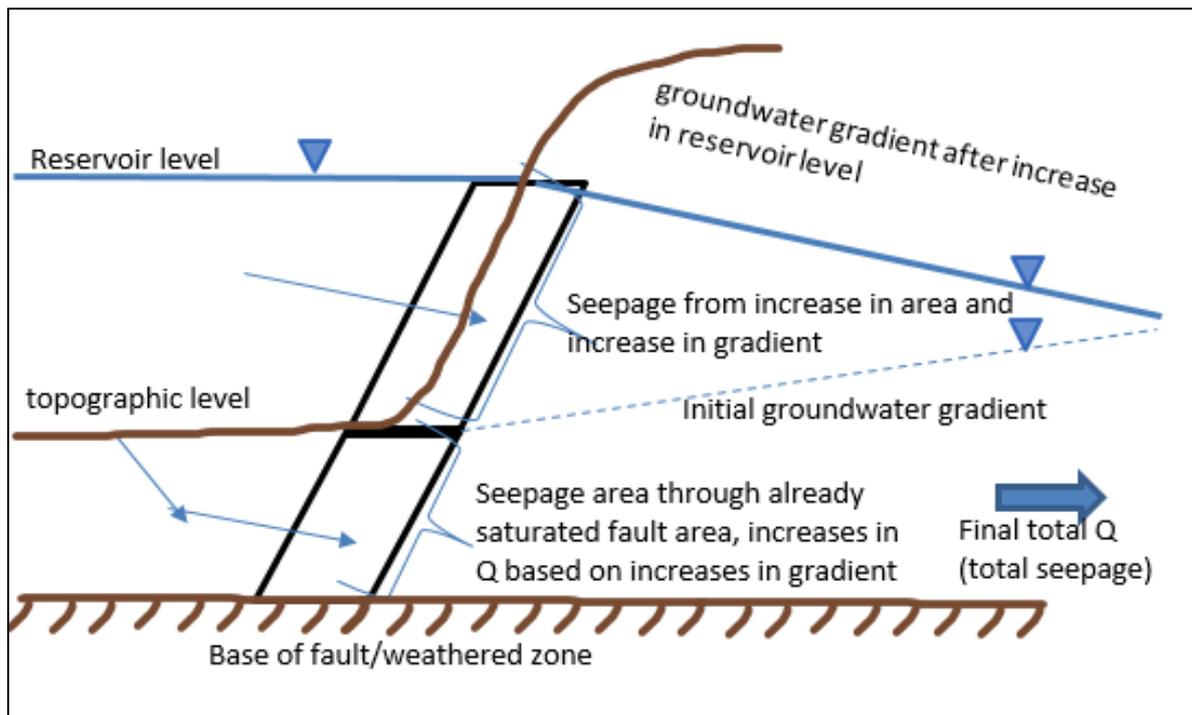
Figure 1-4: Conceptualisation of seepage through faults along eastern fault zone
