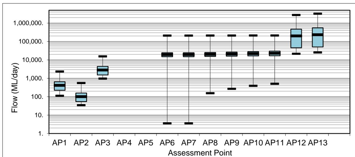
**Figure 4-11: Daily average flow statistics at assessment points post closure with hydroelectric power terminated and all flow through the closure spillway (FRGCP years 34–54)**
