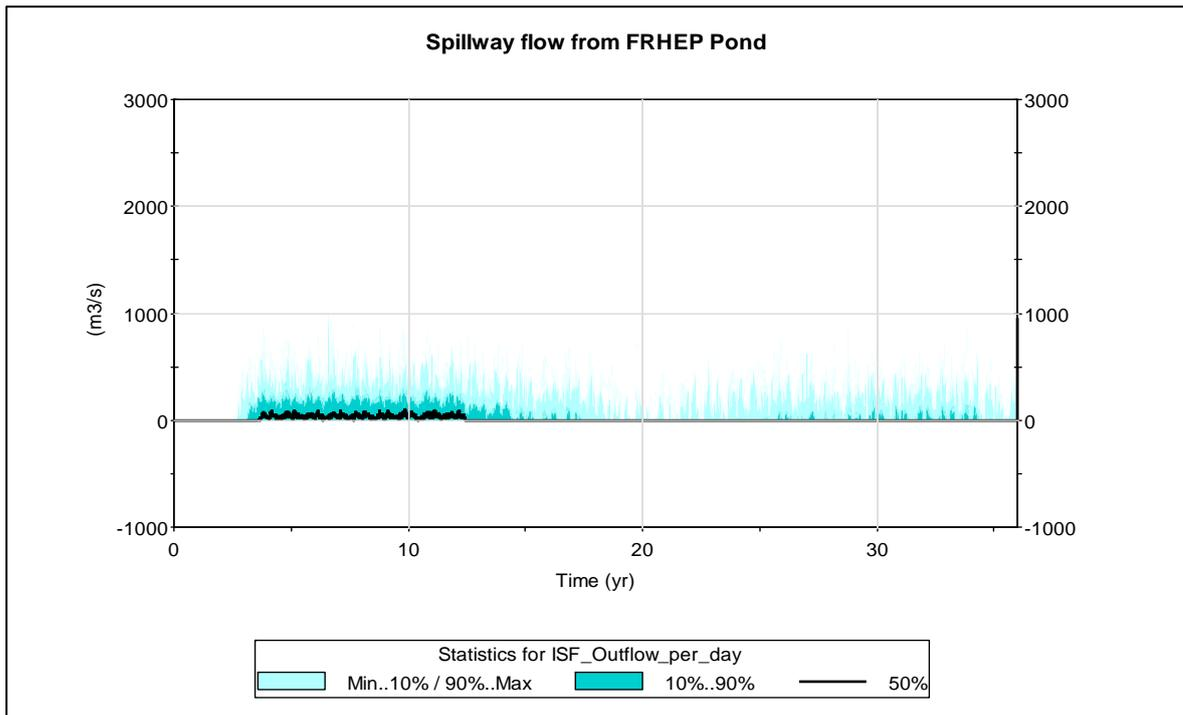
**Figure 4-4: ISF spillway flow – operational period (Model year 0-36, FRGCP year -2 to 33 plus 1 year post FRGCP operations)**
