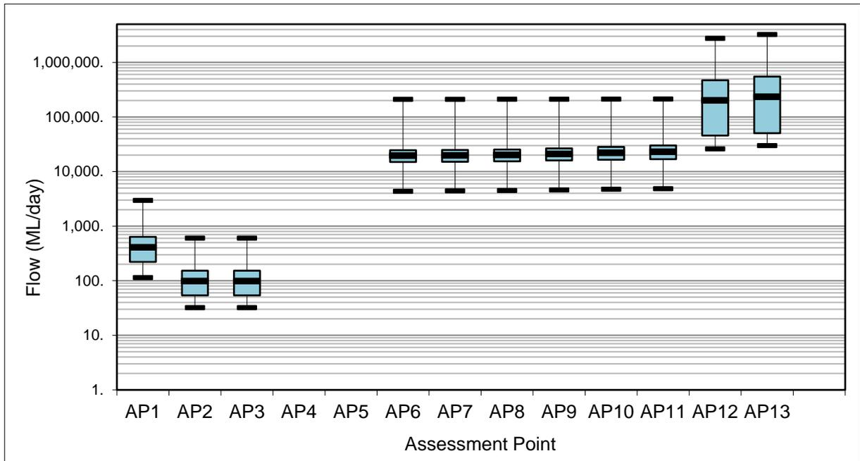
**Figure 4-12: Daily average flow statistics at assessment points post closure with hydroelectric power terminated and environmental flows maintained (FRGCP years 34–54)**
