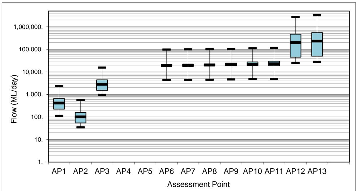
**Figure 4-10: Daily average flow statistics at assessment points post closure with hydroelectric power operations maintained (FRGCP Year 34–54)**
