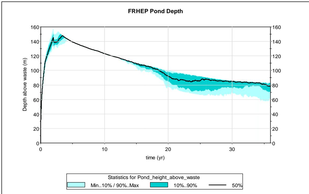
**Figure 4-6: Modelled ISF water depth (above solids) – operational period (Model year 0-36, FRGCP year -2 to 33 plus 1 year post FRGCP operations)**
